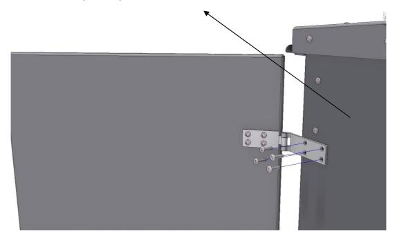
**Step 7:**Mount the lock-mechanism to the door.
