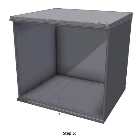
Mount the 4 support brackets that give the Cargo box it's strength.
