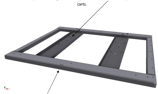
This hole is for the lock-mechanism's conductive strips, and this side is the backside.
