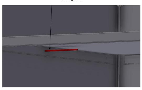
Now remove the shelf so you can drill the marked location of the holes true the side- and back-plate.
