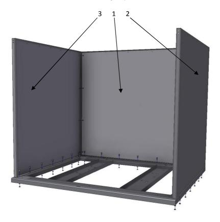
Use M6\*12 bolts, nuts and washers to bolt the side and back of the Cargo-box to the frame.
