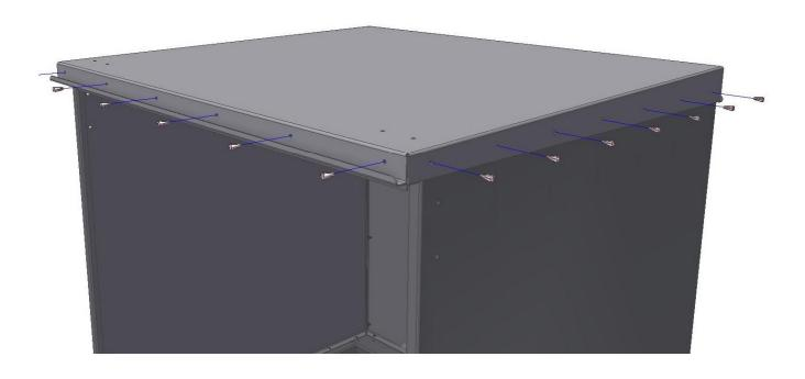
**Step 4:**Mount the bottom plate to the frame as shown on pictures.
