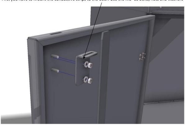
Next is placing the strips that lock the door when the mechanism is finished.
