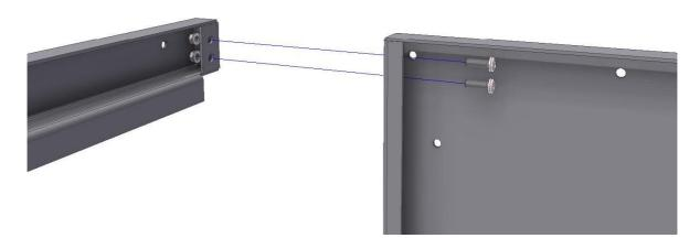
**Step 3:**Mount the top lid to the vertical panels and the support beam.
