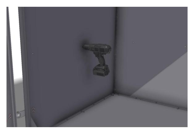
Now you can bolt the shelf into the Cargo-box using bolts, nuts and rivets. Use the M6\*12 bolts, nuts and washers
