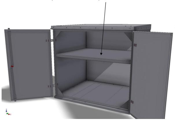
The second thing you need to do is mark the holes of the shelf on the side-panels and back-panel of the cargo box.
