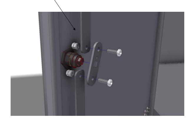
After that you bolt the mounting plate to the lock and the lock-mechanism is finished.
