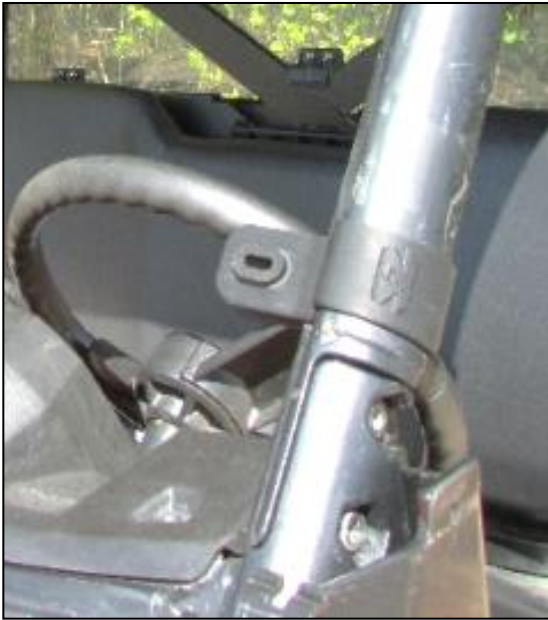
7. Attach the pro-fit roll cage clamps to the vehicle in the approximate location shown.
