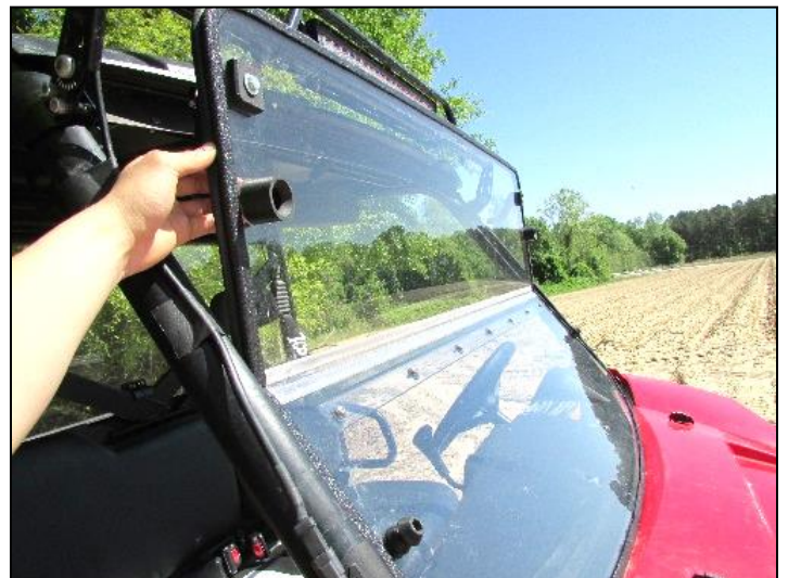
16. Push the top half of the windshield down and firmly press the rubber plugs against each other to lock windshield in down position. (Your vehicle may not be the same as the photo but they work the same).
